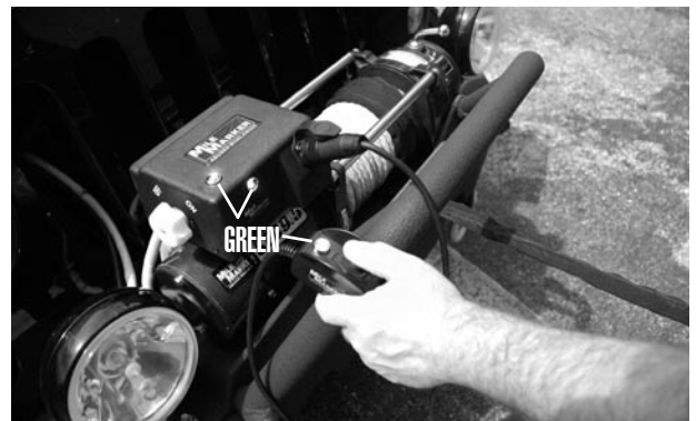
3-8: Toggle Down: Power in, "Green" LED
