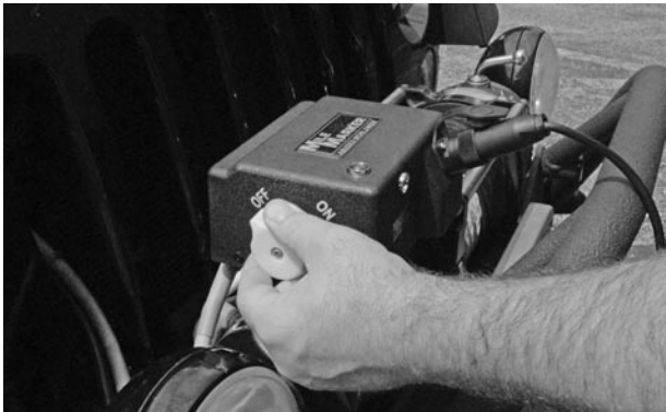
3-5: Rotate Orange Kill Switch from "OFF" position.....
