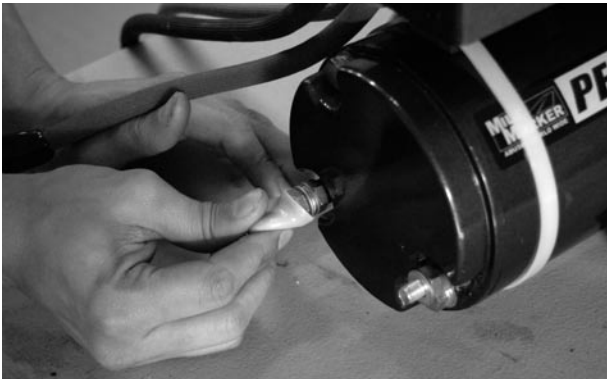
2-11: Cover both stud connections with protective boots.
