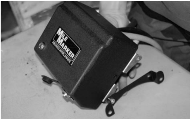
2-2: Remove adaptor bracket from control box with allen wrench and 10mm wrench
